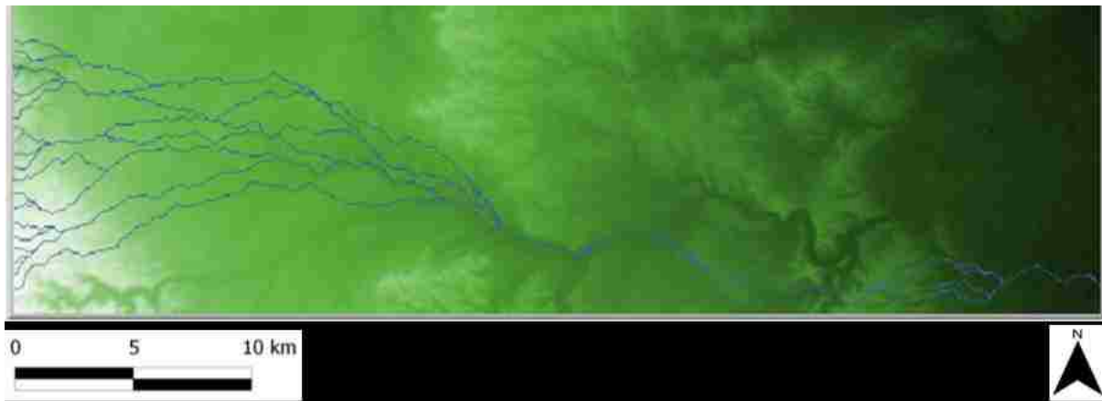
Figure 35: 16 neighbour (Blue) and eight neighbour (Red has been covered over by blue) models.
